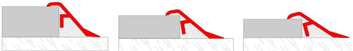
Novonivel® 3 can be installed in three different ways, adapting to three different heights. Ensure the inner wing makes contact with the floor, just as it is represented in the drawing above.
